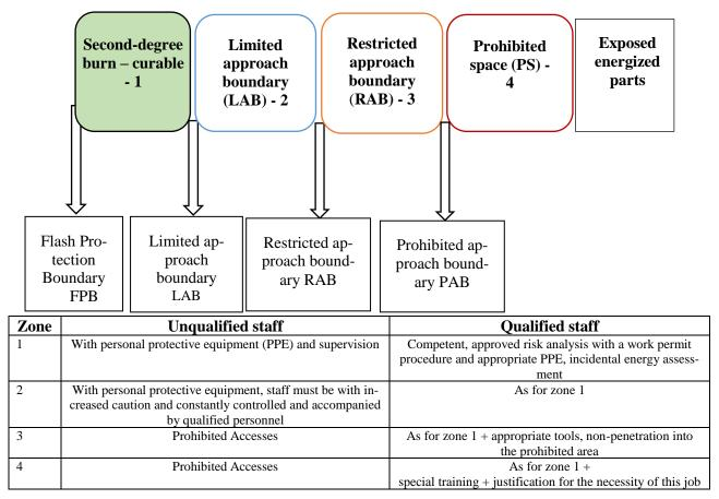
Fig. 1. Boundaries and areas to ensure safety against arc flash risk in accordance with NFPA 70 E (ABB, 2009), (NFPA, 2004).
