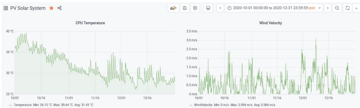
Fig. 10. CPU temperature and wind velocity values from 1 October, 2020 to 31 December, 2020.
