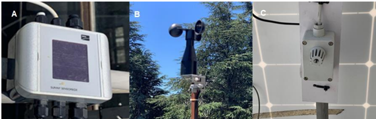
Fig. 2. Measuring System Sunny Sensor Box – A – Solar Radiation Sensor; B- Anemometer; C – Temperature Sensor;
