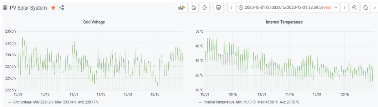
Fig. 9. Grid voltage and inverter temperature values from 1 October, 2020 to 31 December, 2020.
