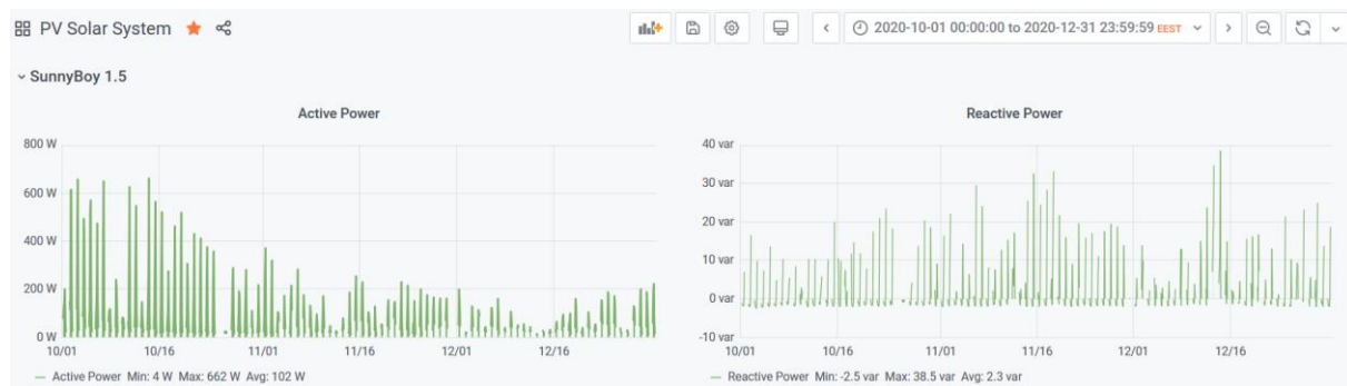
Fig. 5. Active and reactive power values during from 1 October, 2020 to 31 December, 2020.
