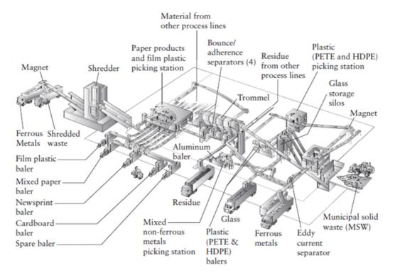
Fig. 9. Typical mixed-waste materials recovery facility (Worrell 2012).
