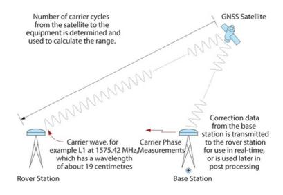
Fig. 1. Principle of operation of RTK.
